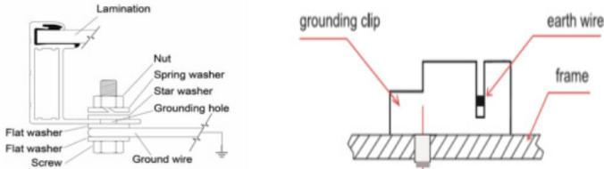
2. Ground using a grounding clamp, as shown below, containing a sliding contact, base and turning tapping screw or 8-32 bolt and hex nut. The grounding clip can hold bare copper wire in the range of 10-12 AWG.
